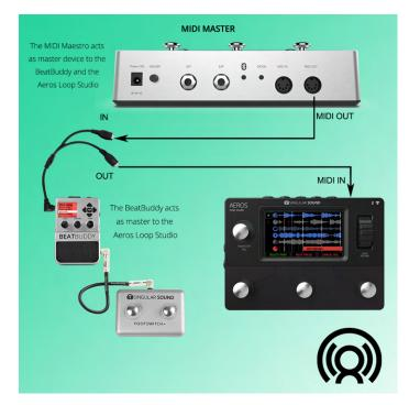
Here is an example of a typical set up using the MIDI Maestro.
